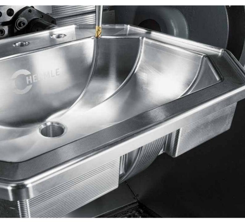
Model making. A hand washbasin for prototyping in aluminum. Highly precise 5-axis simultaneous machining for a perfect finish.
