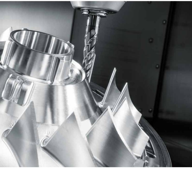
Automotive engineering. Aluminum fan propeller for a tractor engine. After surface reconstruction, the new component is manufactured by means of complex 5-axis simultaneous machining in a single clamping operation.
